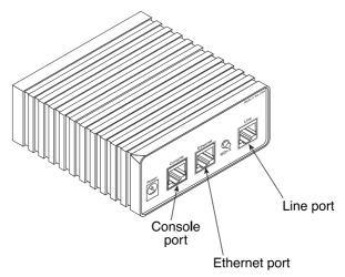
Figure 2. CopperLink Ethernet Extender rear panel
