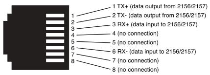
Figure 4. CopperLink Ethernet Extender 10/100Base-T RJ-45 Connector Pinout.
