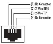
Figure 3. CopperLink Ethernet Extender (RJ-11) twisted pair line interface.
