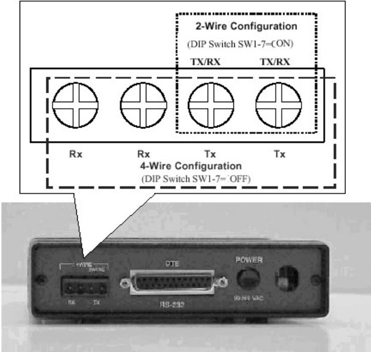
**Figure 2-3. Transmission Line Interface**
