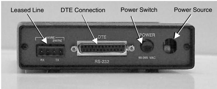
**Figure 2-1. Back View of Modem**
