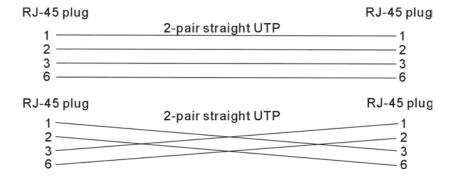
It is suggested to use straight-through UTP cables for all UTP connections. The maximum length and UTP cable categories used for the connections to a 10BASE-T device and 100BASE-TX device are:
