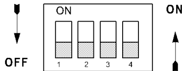
Figure 6. Close-up of DIP Switches Showing "ON" and "OFF" Positions
