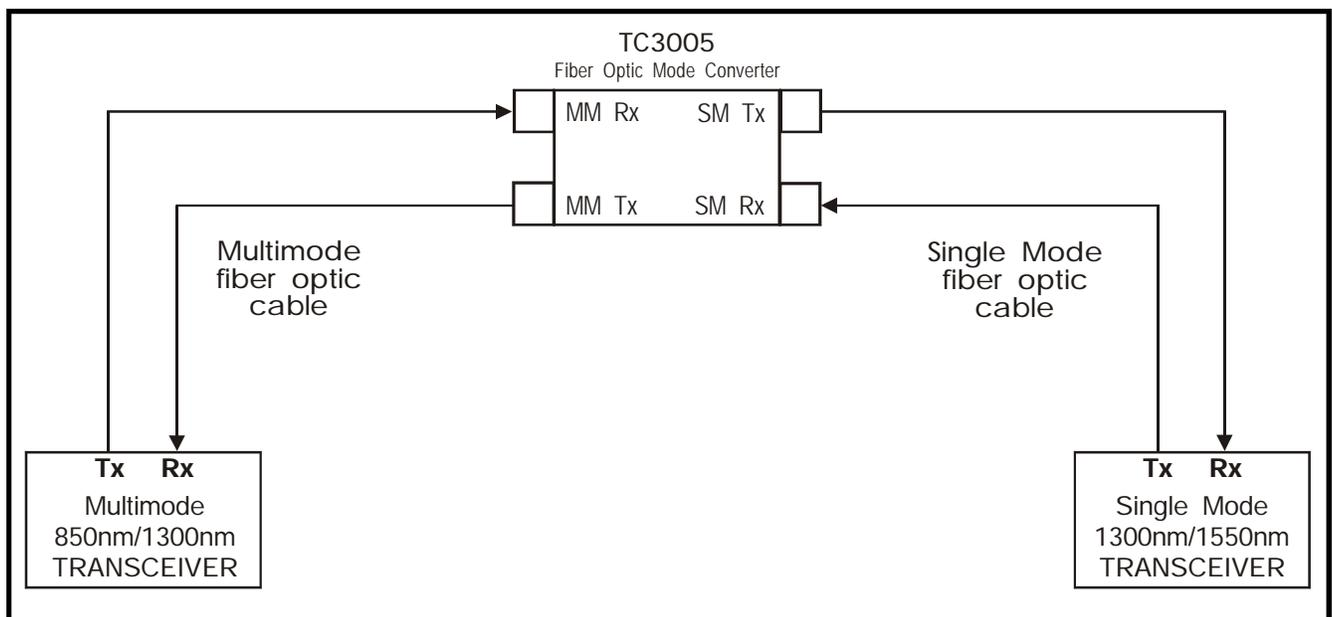
Figure 4. Installation Diagram for Single TC3005 Application
