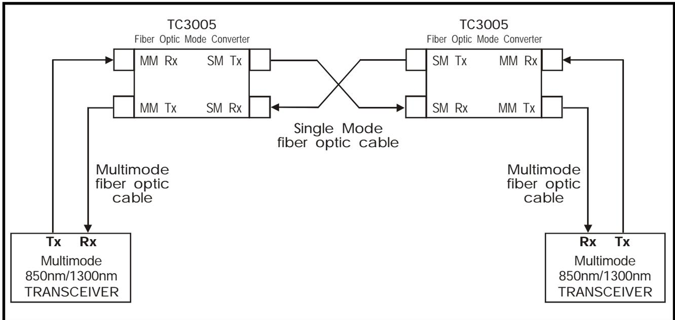
Figure 3. Installation Diagram for Dual TC3005 Application
