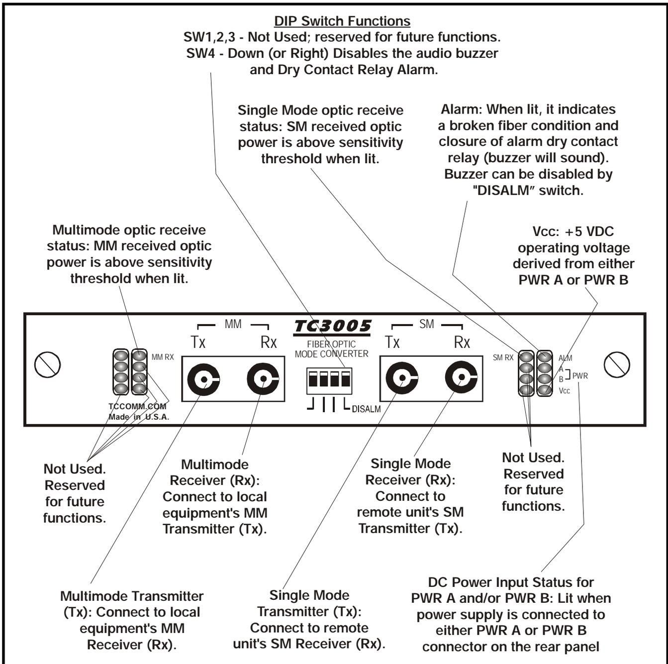
Figure 1. TC3005's Front Panel
