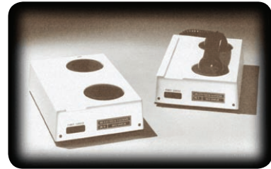
Multi-Tech's first modem, the Acoustic Coupler began shipping in 1971.
